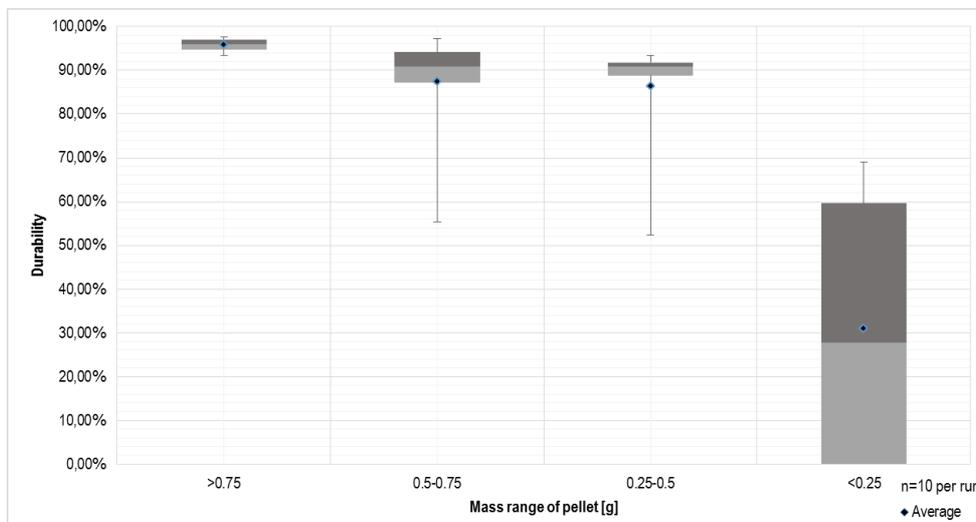
Figure 8 Pellet mass correlation of 60 minutes shaker test
