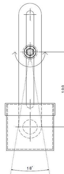
Figure 2 Movement of shaker box
