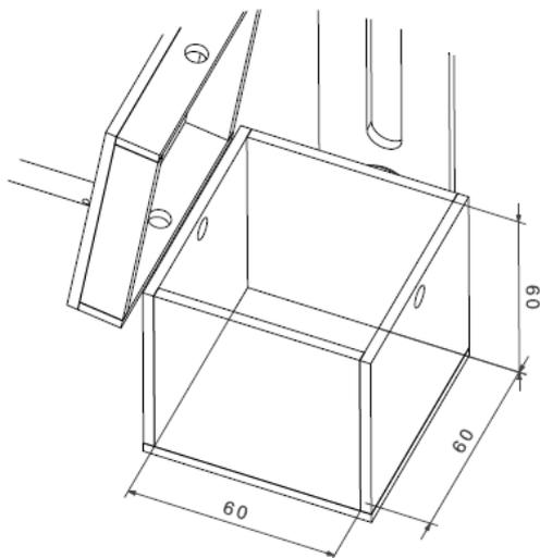
Figure 1 Technical drawing of shaker box
