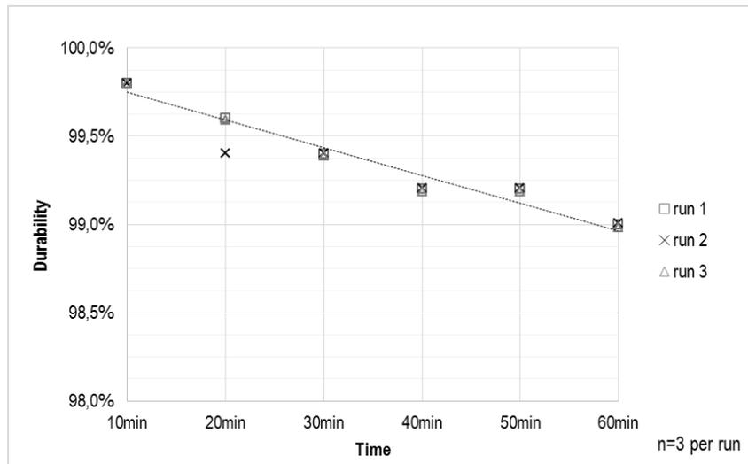
Figure 5 Tumbler durability of sample #1
