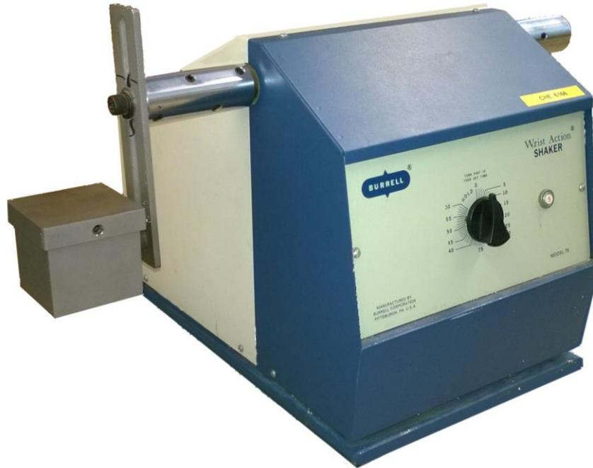
Figure 3 Picture of wrist action shaker with attached durability shaker box
