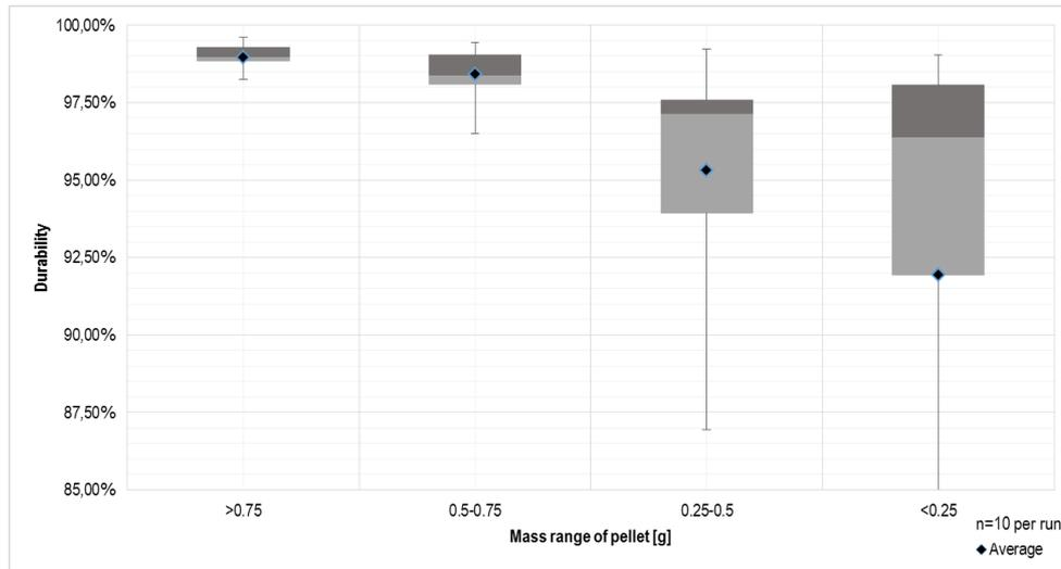
Figure 7 Pellet mass correlation of 10 minutes shaker test
